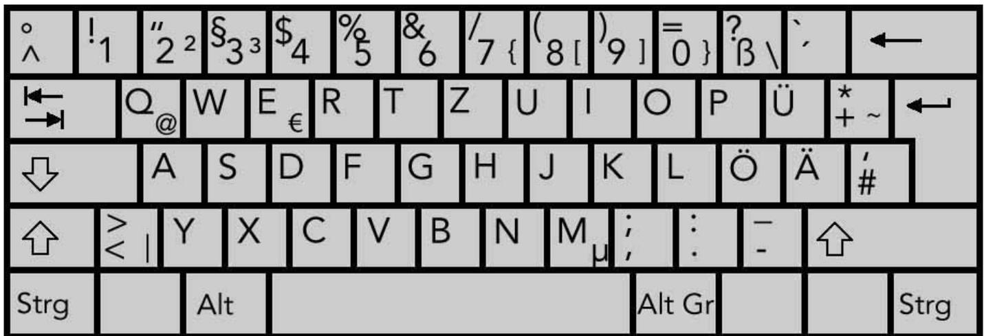
The characters  $^3\{[]\}\ @ \text{€} \mu \sim$  are accessed by holding the **Alt Gr** key and tapping the other key. The **Alt** key on the left will not access these additional characters.
